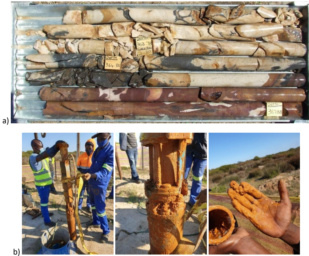
Figure 6— a) Iron and manganese hydrothermal mineralisation within fractured quartzitic sandstones of the Table Mountain Group (TMG) near Cape Town, which results in highly elevated Fe (>30 mg/L) and Mn (>5 mg/L) concentrations within deep fractured TMG aquifer groundwater; b) Iron biofouling from a production borehole within the primary dune sediment Atlantis Aquifer near Cape Town (where iron-coated quartzitic sediment is derived from iron-rich TMG lithology), indicating clogging of pump and water reticulation infrastructure (photos Umvoto Africa).
