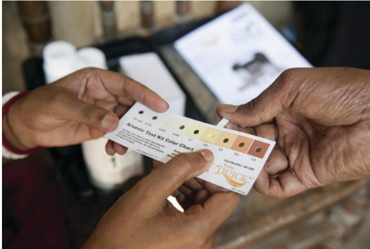
a. Color chart for reading concentration
