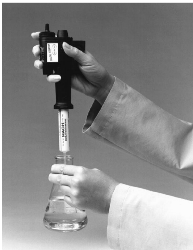
PHOTO 9.1. Digital Titrator for Alkalinity Measurement
