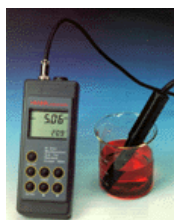
Figure D.4: DO meter with thermistor thermometer
