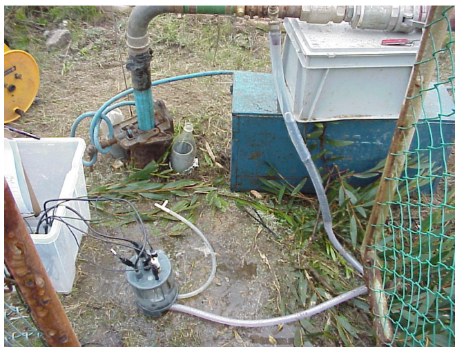
Figure D.1: Measurement of groundwater field parameters using a multiport flow-through cell
