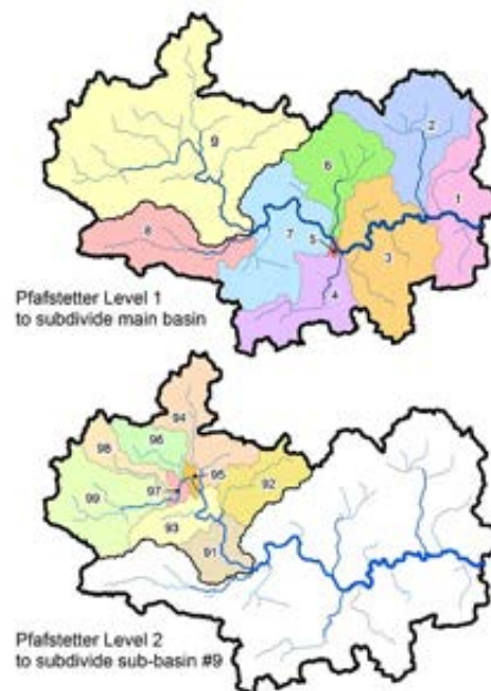
Figure 4 - Example of river basin divided into different levels of sub-basin (from HydroBASINS)
