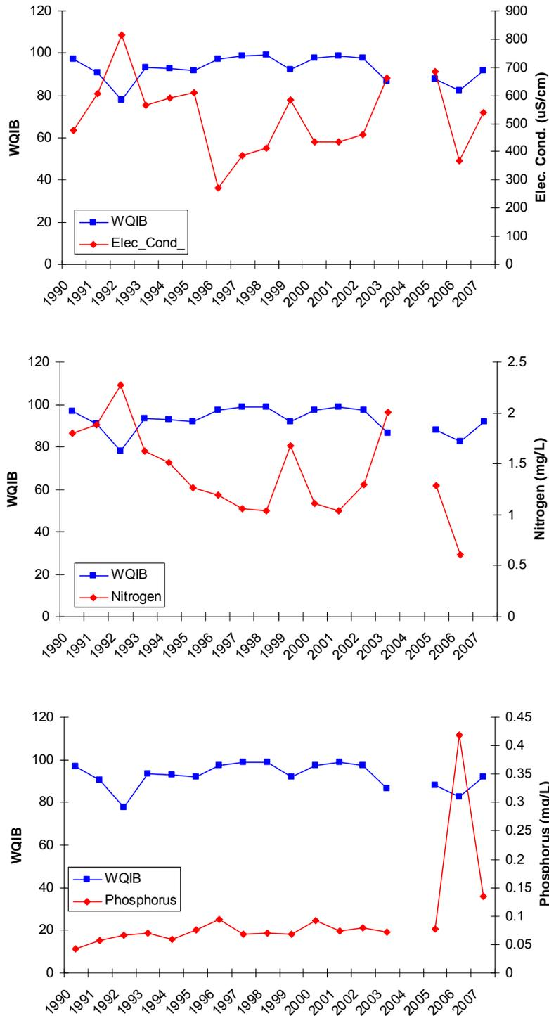
**Figure 9** Water quality index for biodiversity (WQIB) scores and mean annual concentrations of electrical conductivity (top panel), nitrogen (middle panel) and phosphorus (bottom panel) at the Midstream site of the Vaal River, South Africa.
