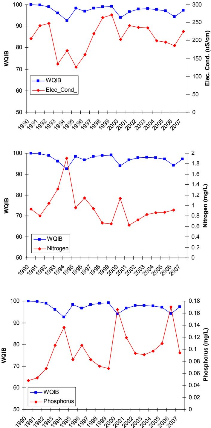
**Figure 7** Water quality index for biodiversity (WQIB) scores and mean annual concentrations of electrical conductivity (top panel), nitrogen (middle panel) and phosphorus (bottom panel) at the Upstream site of the Vaal River, South Africa.
