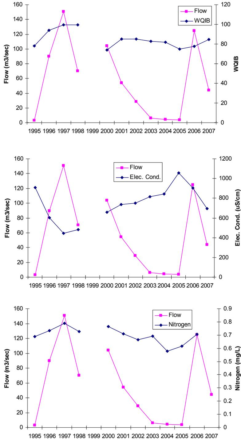
**Figure 14** Flow rates (m<sup>3</sup>/s) against WQIB, nitrogen and electrical conductivity at the Downstream (038003) site in the Vaal River, South Africa.
