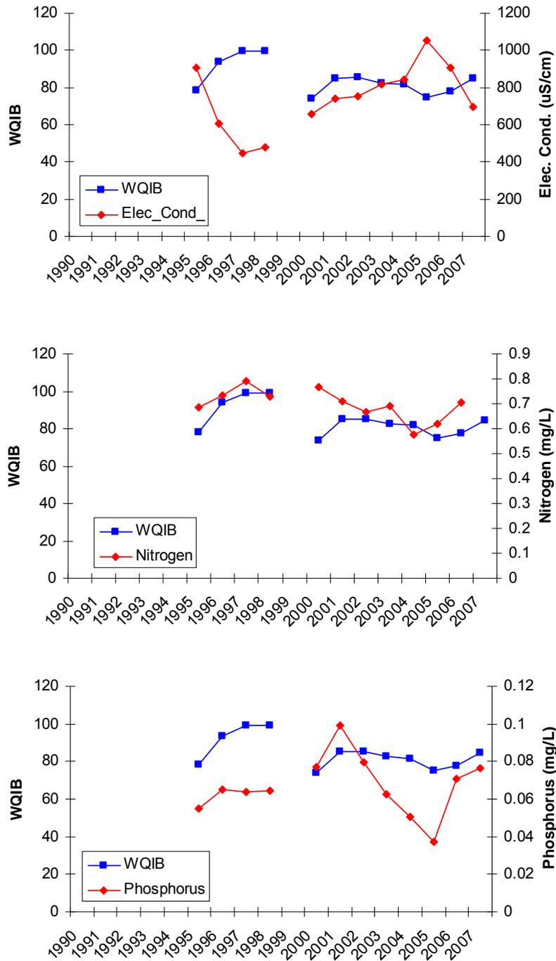
**Figure 10** Water quality index for biodiversity (WQIB) scores and mean annual concentrations of electrical conductivity (top panel), nitrogen (middle panel) and phosphorus (bottom panel) at the Downstream site of the Vaal River, South Africa.
