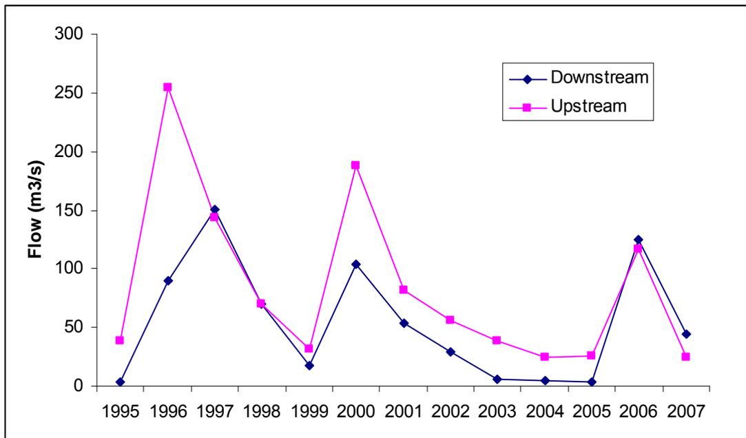
**Figure 12** Flow rates (m<sup>3</sup>/s) at the mid to upstream site (038004) and downstream site (038003) along the Vaal River, South Africa, between 1995 and 2007.
