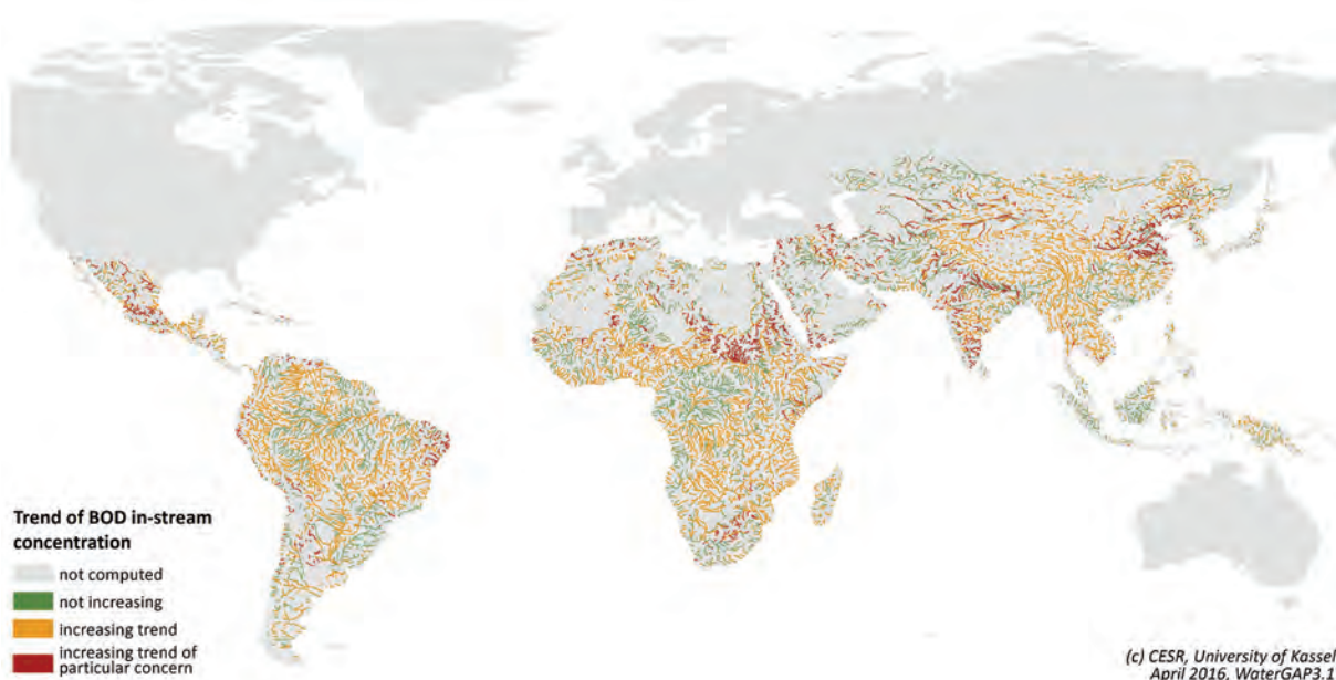
Figure 3.15: Trend in BOD concentrations in rivers between 1990–1992 and 2008–2010. River stretches marked with orange or red have increasing concentrations between these two periods. River stretches marked with red have an “increasing trend of particular concern” meaning that in these stretches the pollution level increased into the severe pollution category in 2008–2010, or that they were already in the severe pollution category in 1990–1992 and further increased in concentration by 2008–2010.
